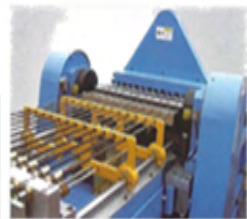
12 tubes can be Bent at one time
