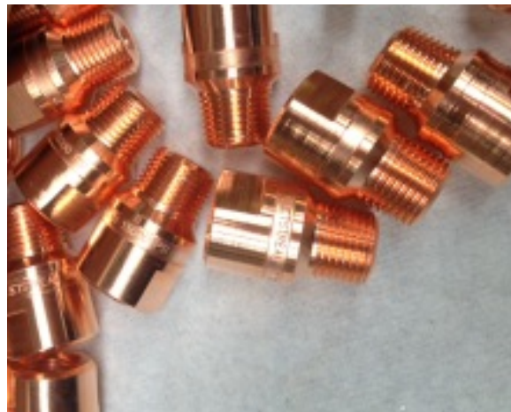
Steel part with a Copper Coating
